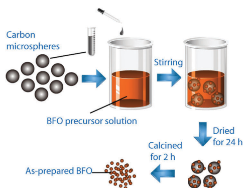
Fig. 1 Schematic illustration of the synthesis of the samples via a carbon microsphere-assisted sol-gel method.
