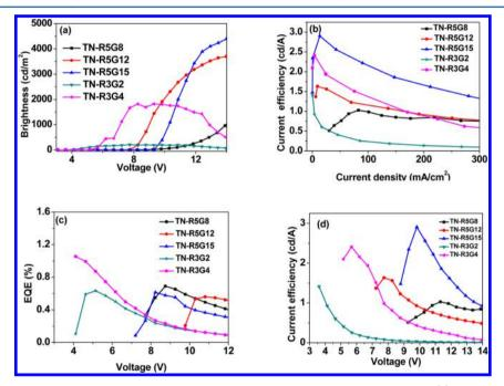
**Figure 4.** EL characteristics of TN-RxGy with the configuration of ITO/PEDOT:PSS/polymer/TPBI/LiF/Al: (a) brightness-voltage characteristics; (b) current efficiency-current density characteristics; (c) EQE-voltage characteristics; (d) current efficiency-voltage characteristics.
