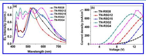
Figure 3. (a) EL spectra and (b) voltage-current density of the devices based on TN-RxGy.
